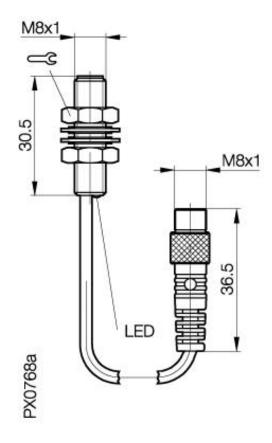
**Inductive Sensors** BES 516-377-G-E4-C-S 49-00,2 M8x1 x 30 normally-closed Sn=2mm shielded
